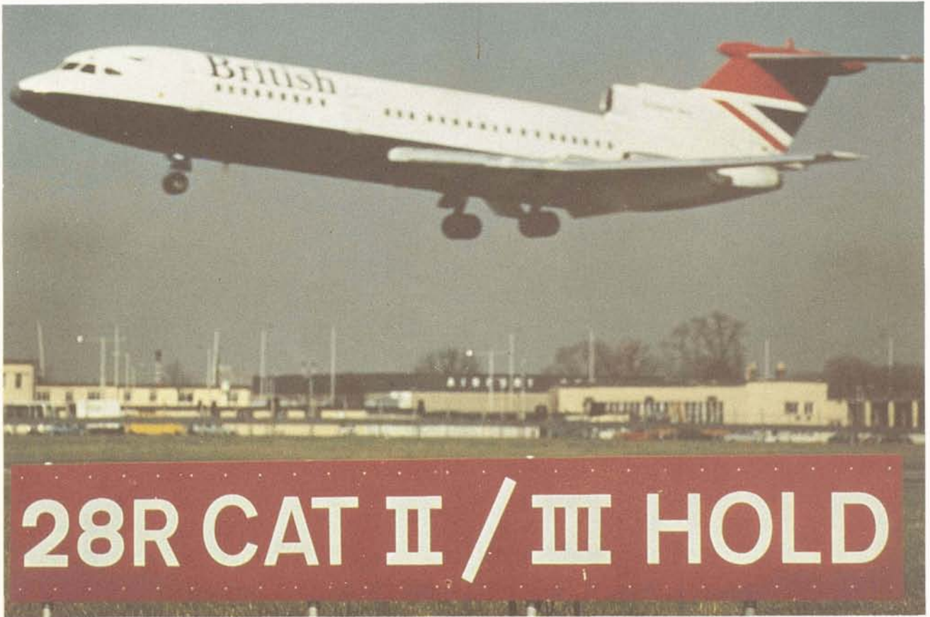
Figure A-3. A Category II/III holding position sign
