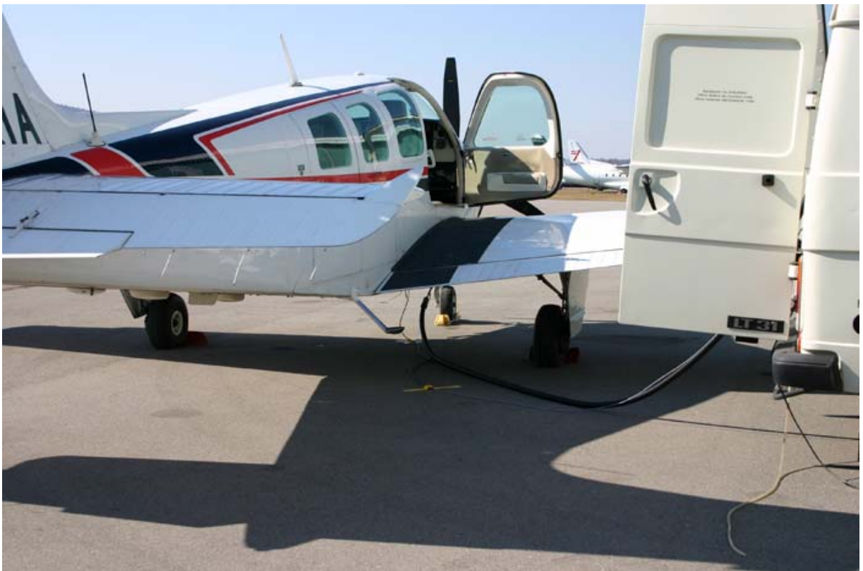
Picture 3: Preparations for ground static emission measurements of HB-KIA
