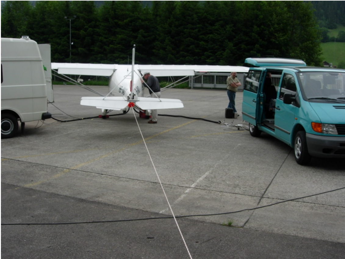
Picture 5: Emission measurement of a Microlight (Swiss Ecolight) aircraft, normally used for glider towing. The power to weight ratio of this aircraft is such that the towing rope is necessary to hold the aircraft in position during full throttle operation.
