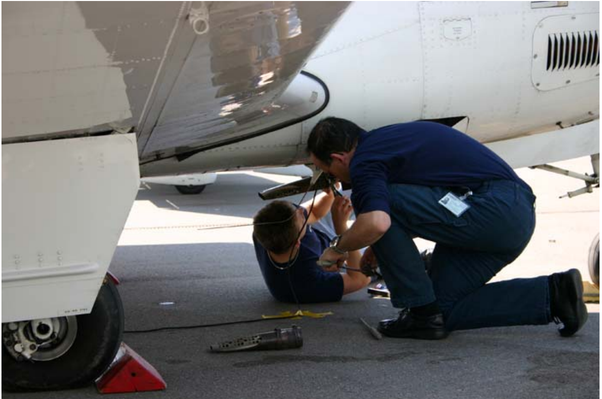
Picture 2: Preparations for ground static emission measurements of HB-KIA
