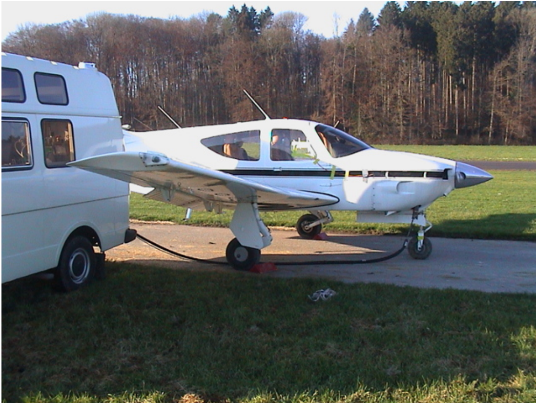
Picture 4: Determination of maximum fuel flow (static measurement). The aircraft brakes are fully applied and the wheels secured by wheel chocks.
