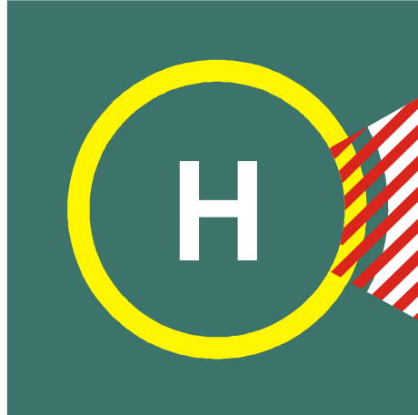
Figure 5-7. Helideck prohibited landing sector marking
