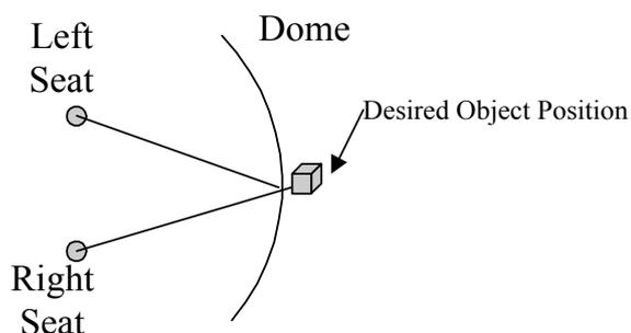
Figure 5 - Near field object in a dome display
