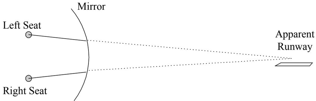
Figure 2 - Runway view in a collimated display
