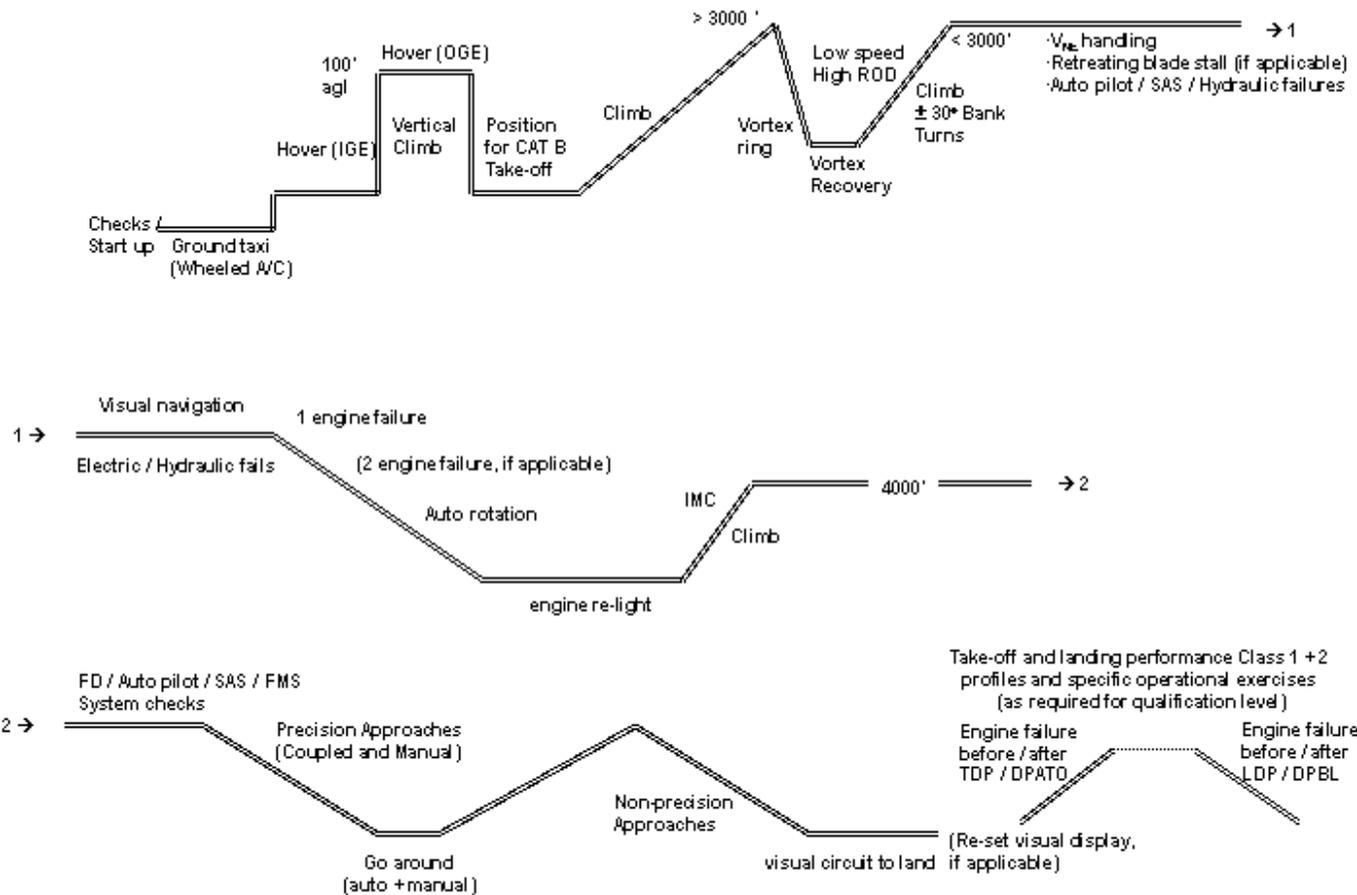
Note: The Typical Test Profile should be flown at helicopter masses at, or close to, the maximum allowable mass for the ambient atmospheric conditions. Those ambient conditions should be varied from Standard Atmosphere to test the validity of the limits of temperature and pressure likely to be required in the practical use of the FSTD. Visual exercises only apply to FSTDs fitted with a visual system.
