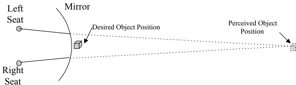
Figure 4 - Near field object in a collimated display
