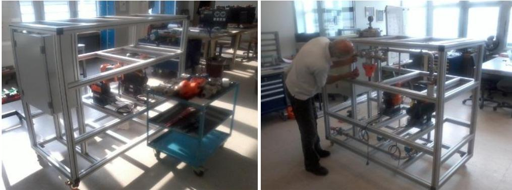
**Figure 6.4. Construction of the fuel doping system in the apprentice shop of SR Technics.**
