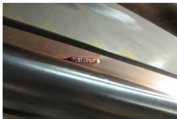
**Figure 6.7. Cracked welding seam on the sampling probe.**
