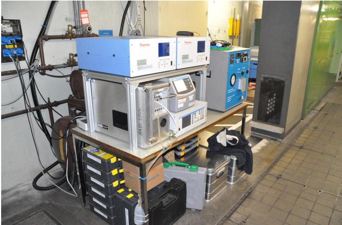
**Figure 2.4. Annex 16 instrumentation for gas analysis and smoke number.**
