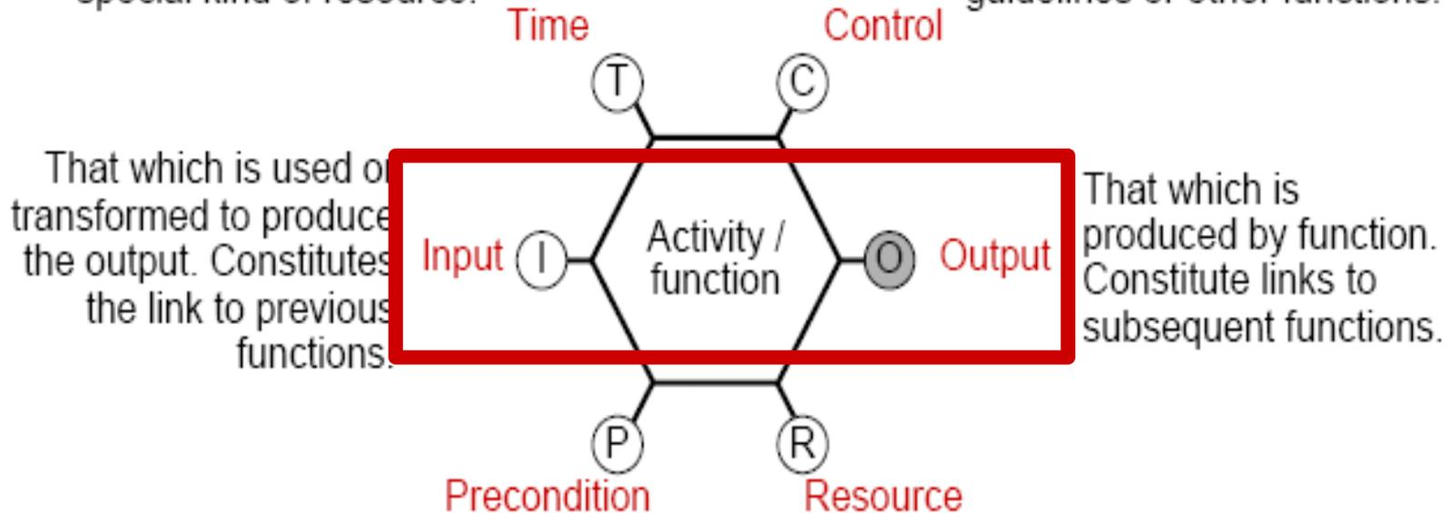
That which is used or transformed to produce the output. Constitutes the link to previous functions.
