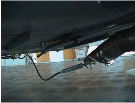
Picture 4: Exhaust probe
