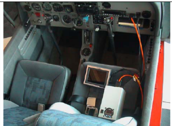
Exhaust tester: view from baggage boot door
