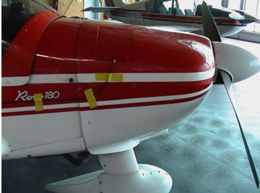
Picture 1: Electronic RPM and fuel flow installation
