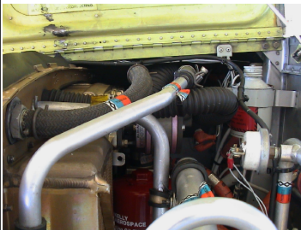
E) RPM sensor signal line (black, from left top to right bottom)
