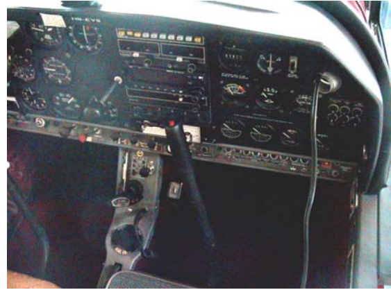
Picture 5: Cockpit of HBEYS with 12VDC/70W power supply for the gas analyzer on the right.
