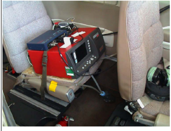
B) Installation of Stargas898 unit (total Mass 10 kg)
