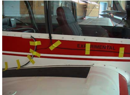
Picture 2: Sampling lines in and out
