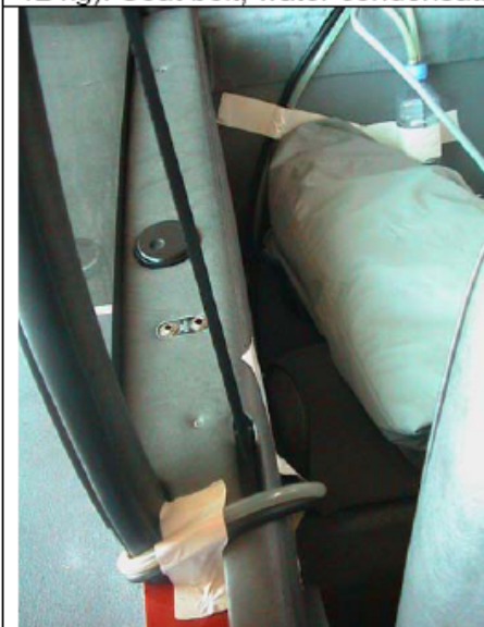
Exhaust lines: incoming (black) and outgoing (transparent). The cockpit door (canopy) stays 2 cm open during flight.
