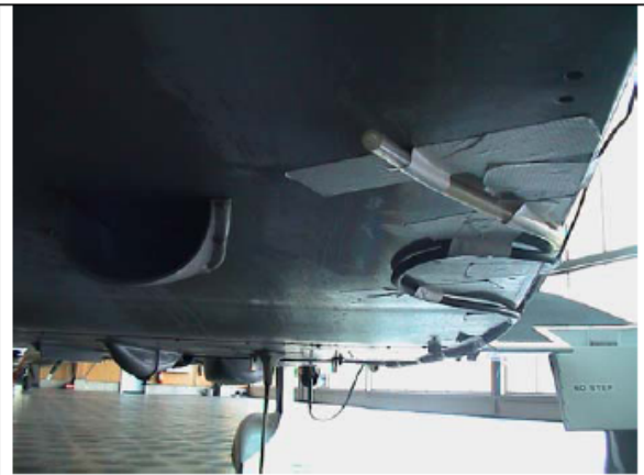
Exhaust line: incoming and outgoing lines to and from measurement equipment
