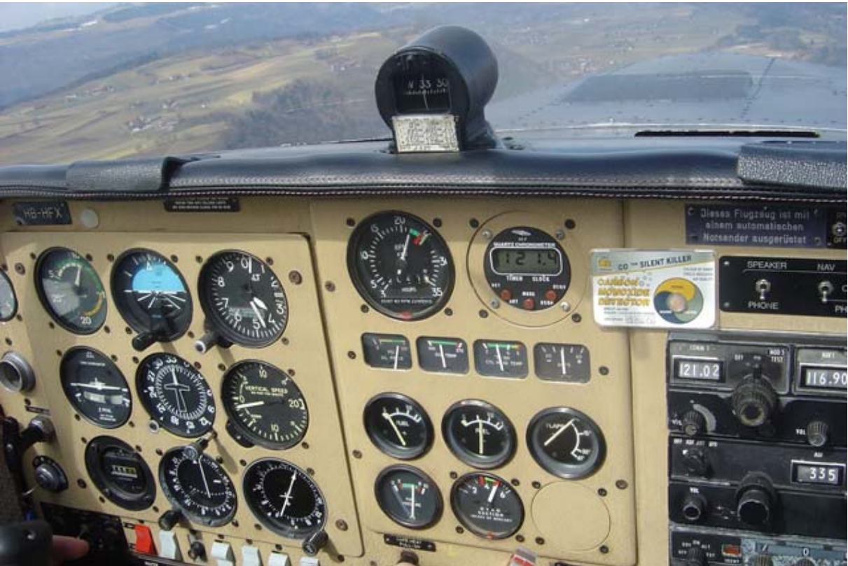
Picture 10: HBHFX cockpit during measurement flight with cabin CO-detector (right hand side)
