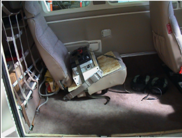
A) Installation of Battery (total Mass 25 kg)
