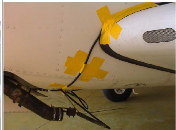
F) RPM signal line and exhaust probes
