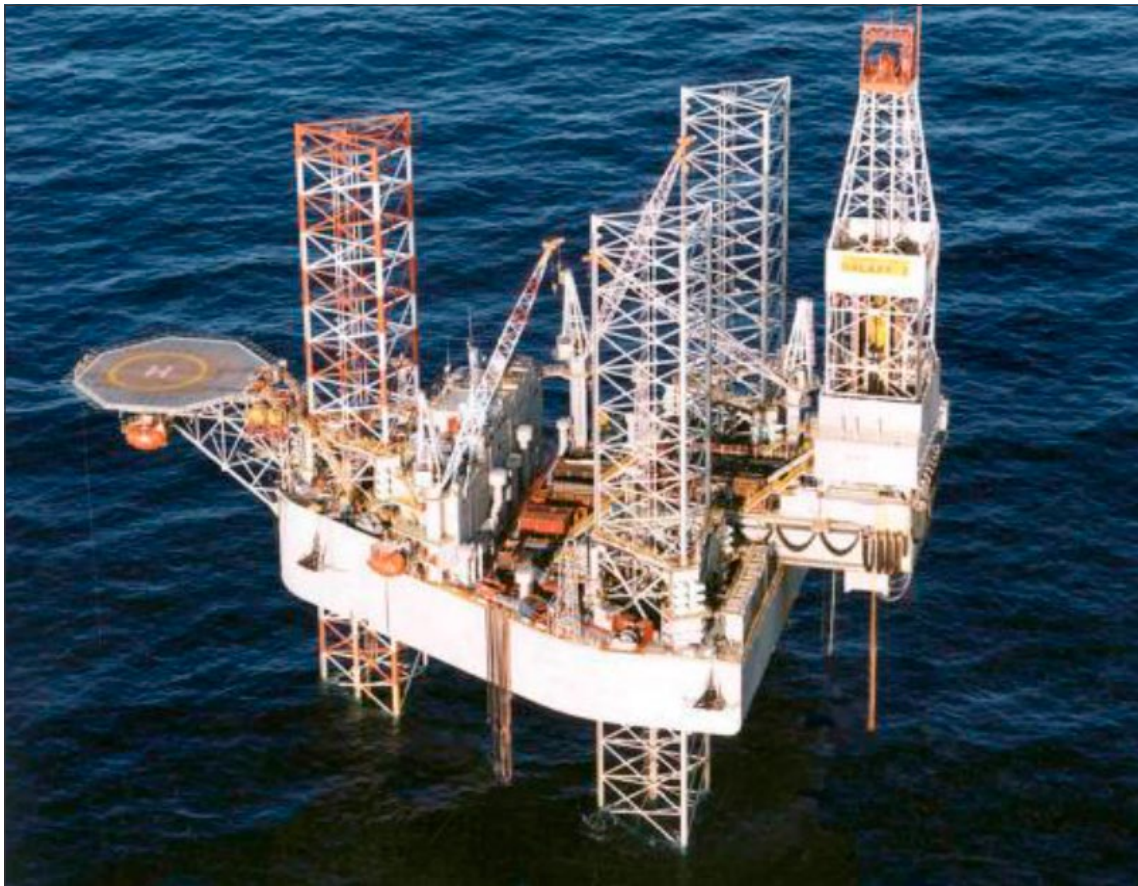
Figure I-1-3. A three-legged jacked-up mobile offshore drilling unit
