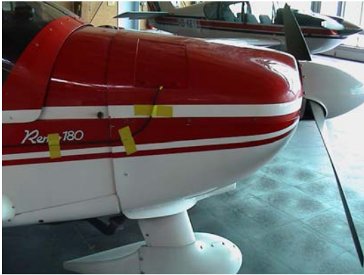
Picture 1: Electronic RPM and fuel flow installation
