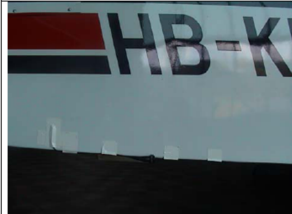
Temperature probe: fixation on right side of fuselage
