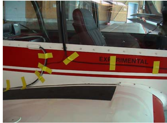
Picture 2: Sampling lines in and out
