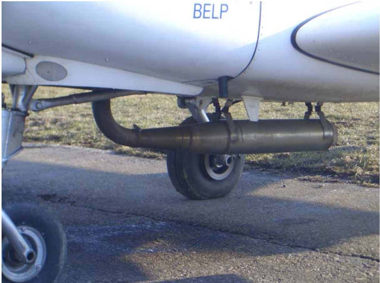
Picture 8: HB-HFX with original exhaust muffler (Gomolzig).
