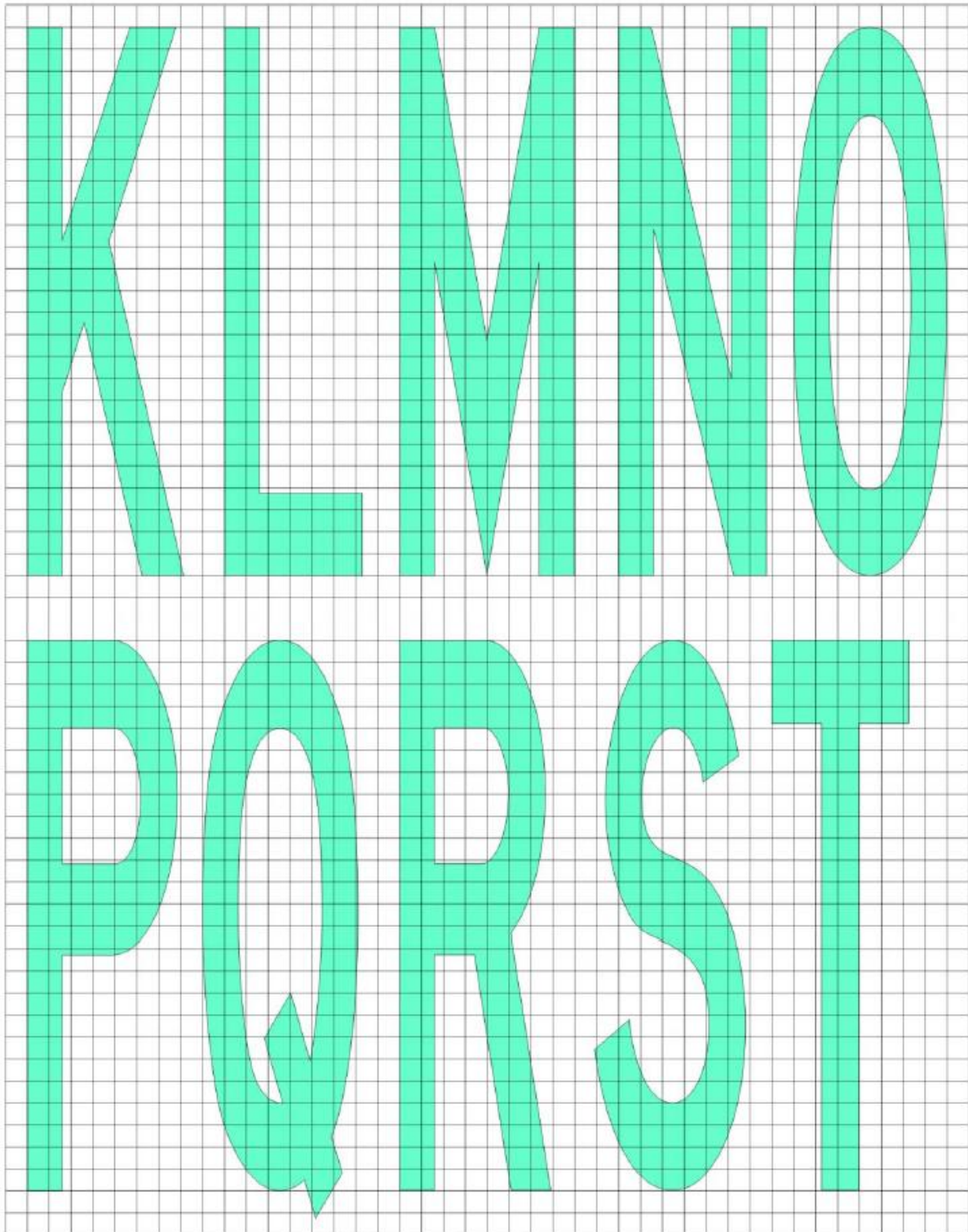
Figure L-10B. Mandatory instruction marking inscription form and proportions
