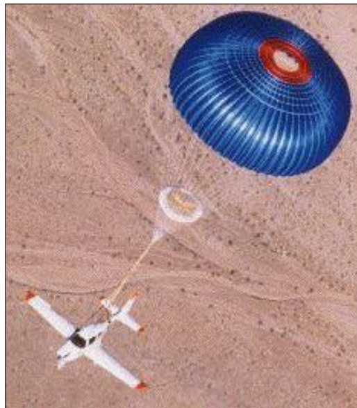
Figure 2-2. Rocket-deployed emergency parachute system
