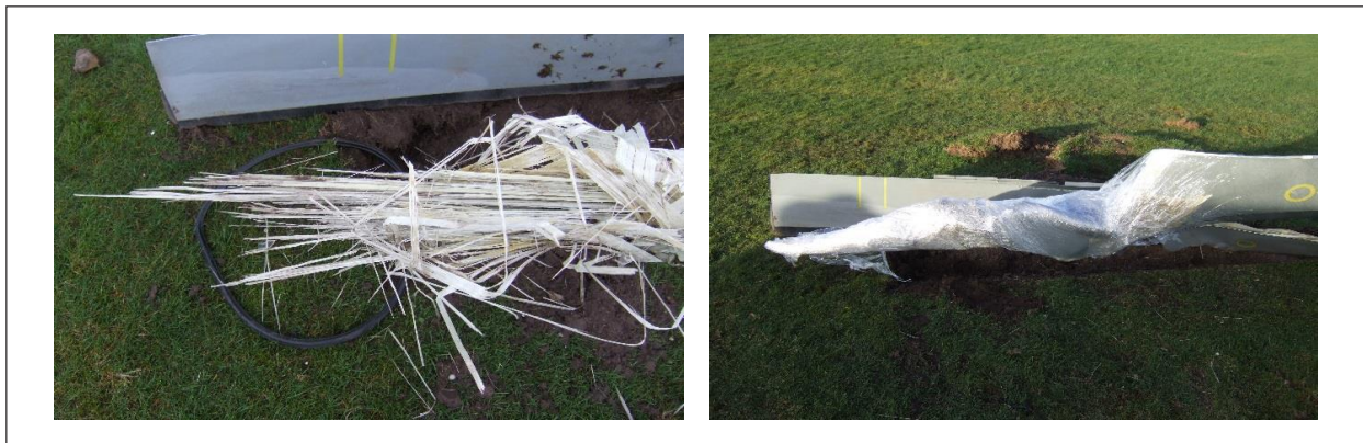
Figure 2-6. “Wrapping” rotor blades to reduce contact hazards
