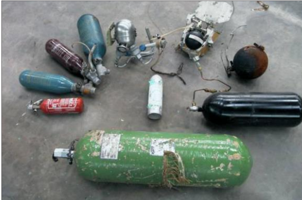
Figure 2-1. A selection of pressurized containers recovered from aircraft accidents
