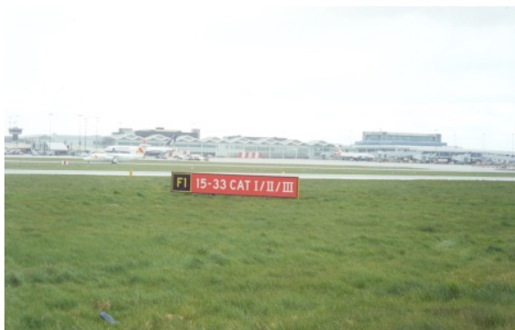
Figure 12-7. Examples of typical sign designs
