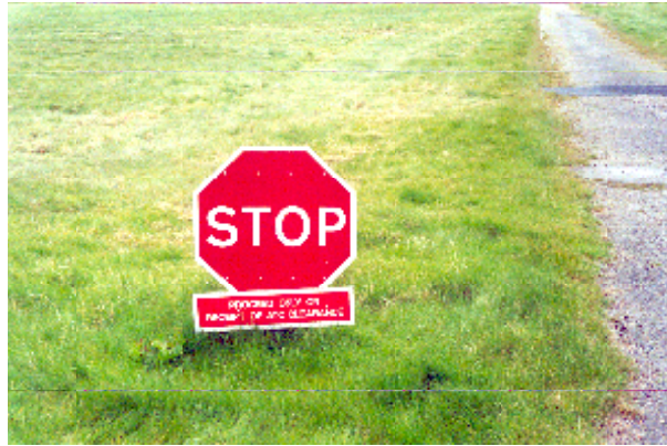
Figure 12-4. Road-holding position sign
