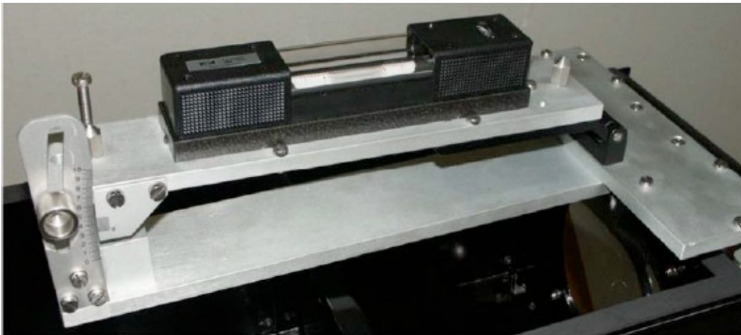
Figure 8-12. Spirit level clinometer Photo source: ADB Safegate
