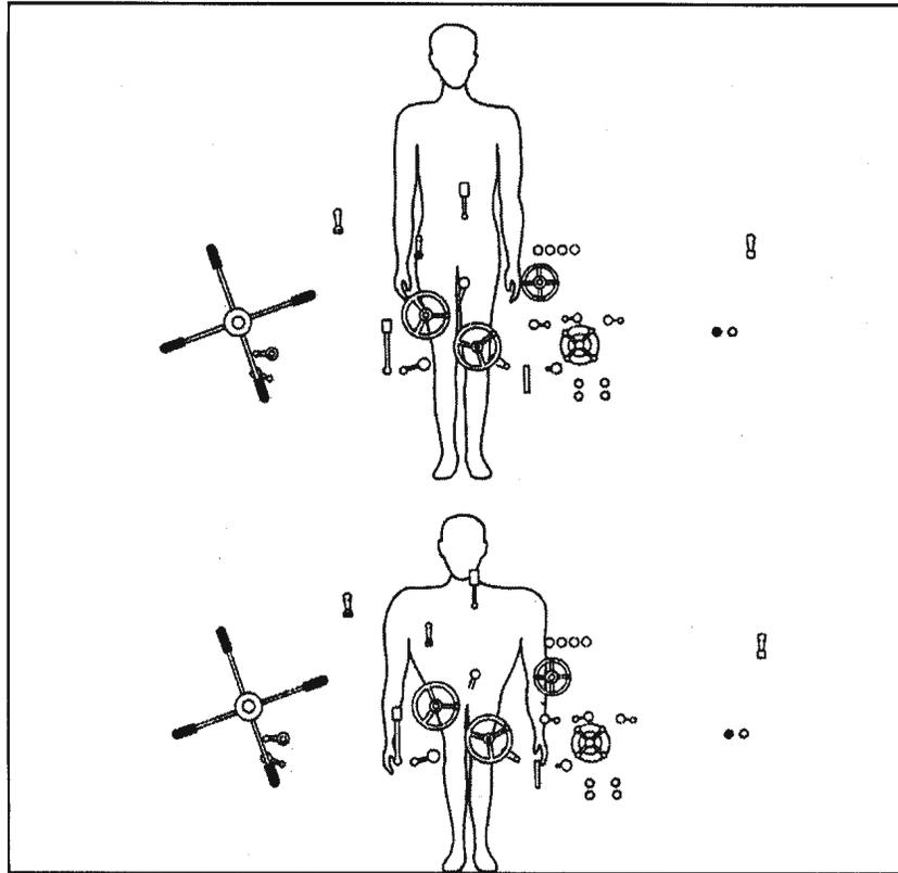
**Figure 4-5. The controls of a lathe in current use are not within easy reach of the “average” person**
