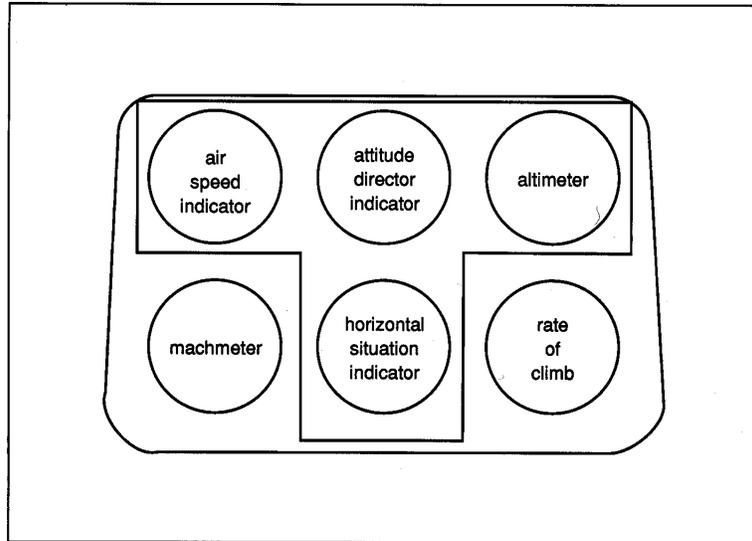
**Figure 4-13. The “basic T panel” which forms the core of modern flight instrument panel layouts**
