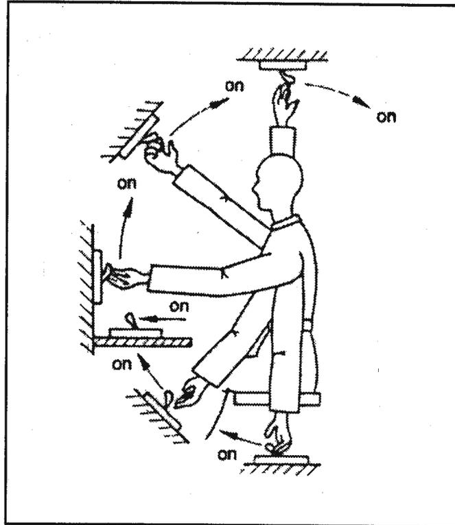
**Figure 4-16. The “sweep-on” switch position concept which is slowly replacing the earlier “forward-on” arrangement**
