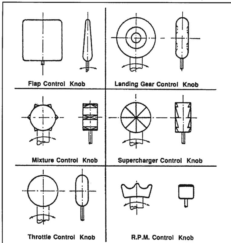
Figure 4-8. FAA requirements for cockpit control knobs
